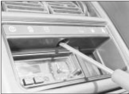
23.7 Remove the screw from the warning lamp fascia panel
