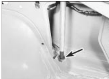
53.4 Pull the base of the aerial from the rubber bush (arrowed)
