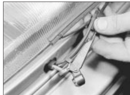
32.4 Removing a headlamp wiper arm
