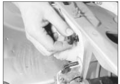
42.5 Adjusting the headlamp alignment
