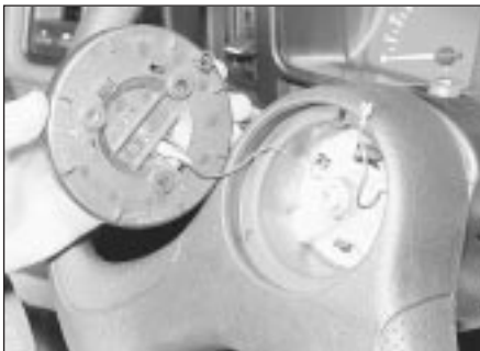
11.6 Prise the trim insert from the steering wheel, followed by the centre disc - models from 1987
