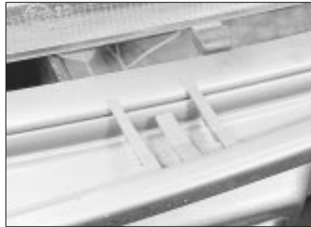
40.5a Prise the trim strip from the bottom of the headlamp unit . . .
