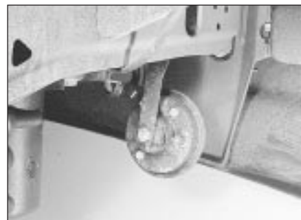
29.1 Horn location beneath front panel
