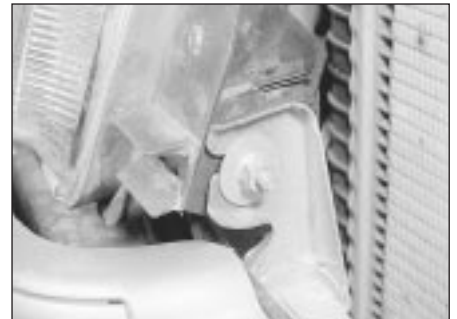
41.10c . . . and the side securing nut - models from 1987
