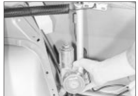
53.5 Removing an electric aerial - Saloon model
