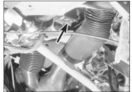
6.3 Direction indicator/hazard warning flasher relay location (arrowed)
