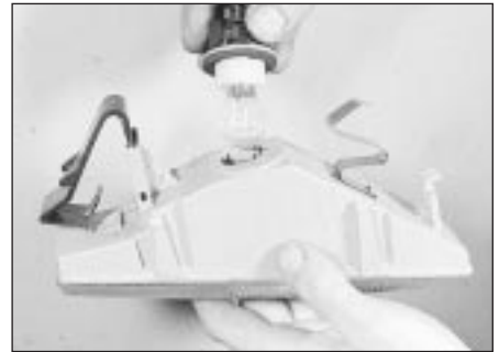
48.15 Removing a front direction indicator lamp bulb - models up to 1987
