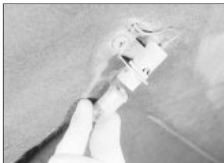
28.6 Removing an underbonnet lamp bulb
