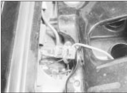
48.9 Withdraw the auxiliary driving lamp bulb from the headlamp unit - models up to 1987
