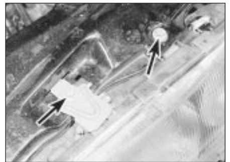
41.4a Remove the upper headlamp securing bolts (arrowed) . . .
