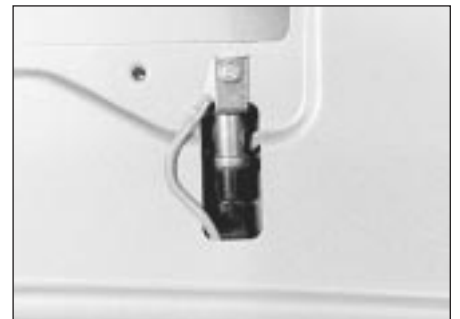
13.4 Luggage compartment lamp switch location - models up to 1987
