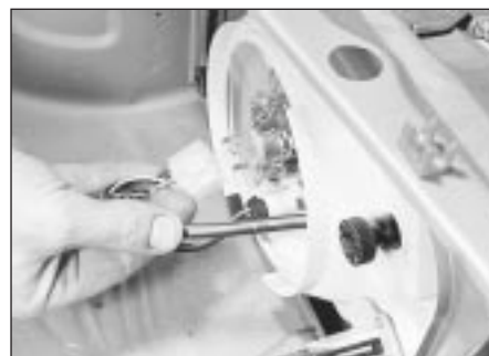
48.3a Pull off the wiring plug . . .
