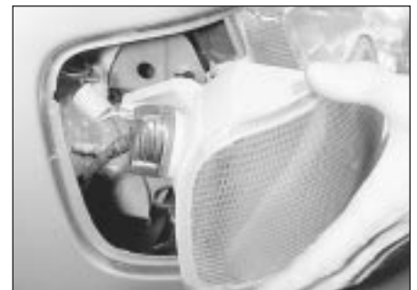
44.8b . . . and withdraw the lamp unit
