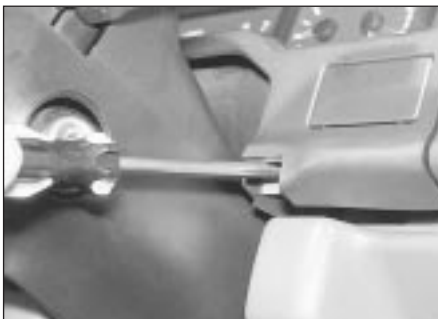
20.11 Removing an instrument panel surround lower securing screw (cover removed)
