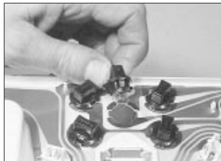
21.3a Removing an instrument panel warning lamp bulb - bulb is a push-fit in the bulbholder
