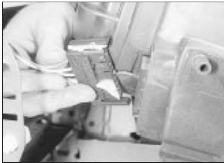
41.8 Disconnect the headlamp wiring plug - models from 1987
