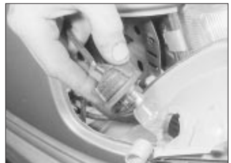
48.18 Removing a front direction indicator lamp bulb - models from 1987
