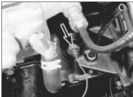
16.2 Oil pressure warning lamp switch location (arrowed) - SOHC engine
