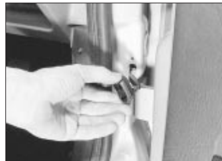
12.3 Withdrawing a courtesy lamp switch
