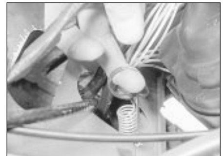
44.8a Unhook the front direction indicator lamp unit anchor spring . . .
