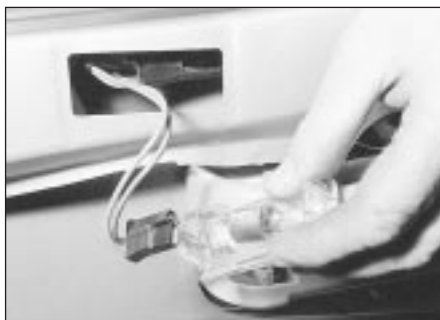
27.24 Removing a luggage compartment lamp bulb
