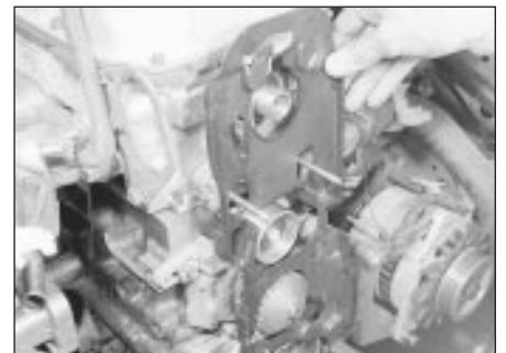
18.13 Removing the timing belt backplate - 1.8 litre (R2A)
