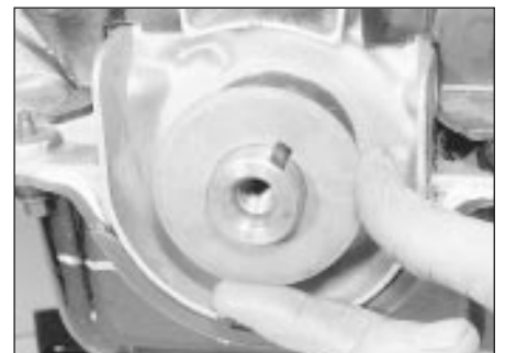
18.10c ... and the thrustwasher - 1.8 litre (R2A)
