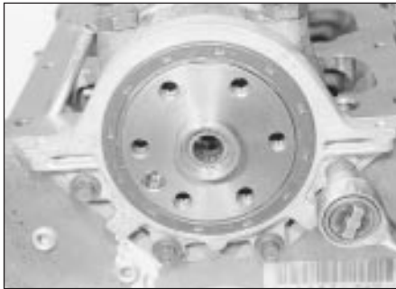
32.25 Fit the crankshaft rear oil seal housing and tighten the securing bolts - 1.8 litre (R2A)
