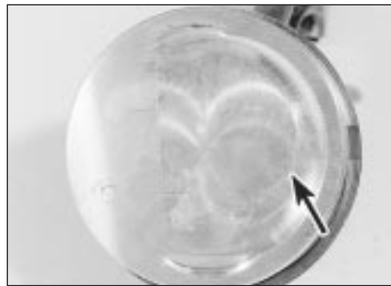
30.10a Cut-out (arrowed) in piston crown . . .
