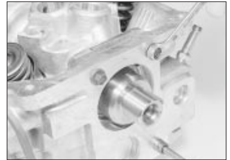
23.11b . . . and tighten the securing bolts - 1.8 litre (R2A)
