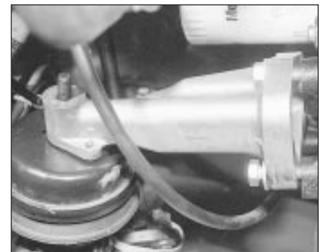
16.6 Locating pin on mounting must engage with hole (arrowed) in engine mounting bracket
