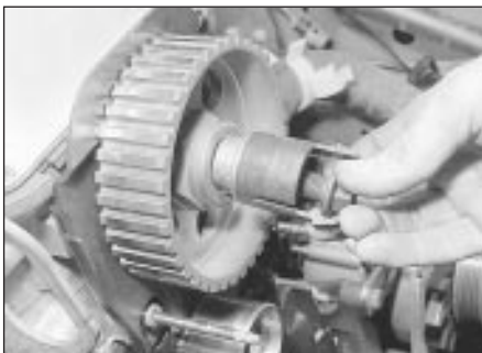
18.11 Removing the camshaft sprocket bolt and distributor rotor shaft - 1.8 litre (R2A)
