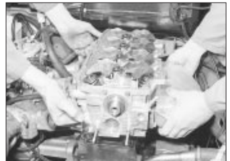
20.6 Withdraw the cylinder head bolts and lift the cylinder head from the block - 1.8 litre (R2A)
