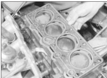
20.7 Recover the cylinder head gasket - 1.8 litre (R2A)
