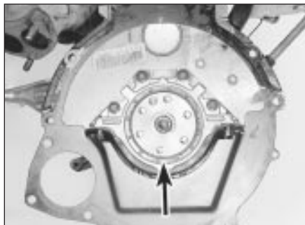
26.2 Crankshaft rear oil seal location (arrowed)
