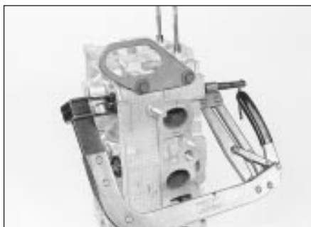
21.2a Compress the valve spring . . .
