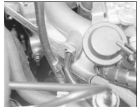
8.9 Disconnecting the brake servo vacuum hose from the inlet manifold - 1.8 litre (R2A)
