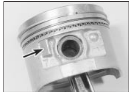
30.10b . . . and lug (arrowed) on piston skirt must face the front of the engine
