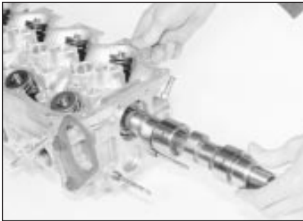
23.10 Refitting the camshaft - 1.8 litre (R2A)
