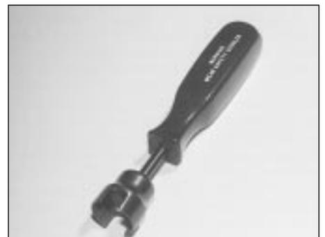
Brake shoe steady spring cup removal tool
