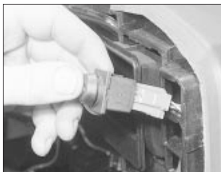
15.54 Removing a foglight switch
