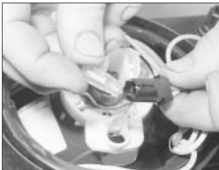
3.8 Removing the front parking light bulb from the holder
