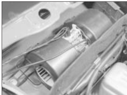
29.5 Blower motor showing wiring connections
