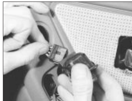
15.15 Removing a mirror control switch
