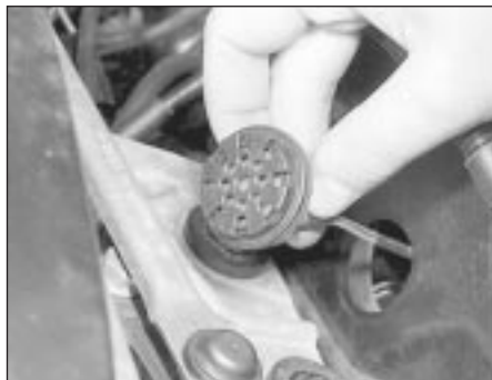
36.9 Removing the alarm system warning buzzer
