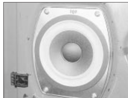
31.4 Front door loudspeaker - note TOP marking
