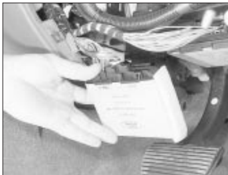
36.6 Removing the anti-theft alarm control module
