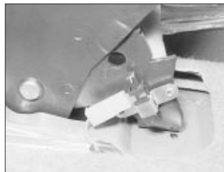
15.39 Handbrake "On" switch
