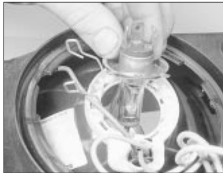
3.3 Removing a headlight bulb
