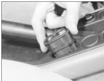
15.31 Removing a window operating switch
