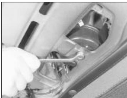
31.8 Removing a rear speaker retaining bolt
