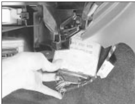
28.10 Removing the speed control module
