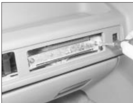
30.19a . . . undo the retaining screws . . .
