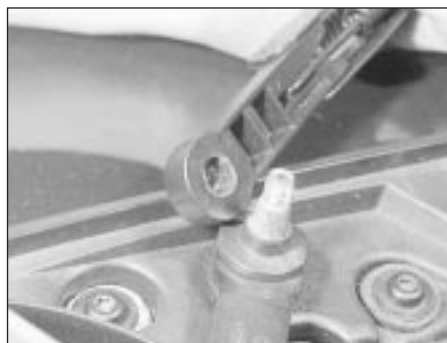
22.3b Pull the arm off the spindle
