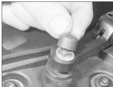
22.3a Lift the cap to expose the nut
