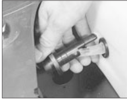
27.19 Removing the washer fluid level switch
