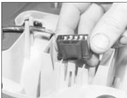
4.13 Disconnecting the multi-plug from the rear light unit
