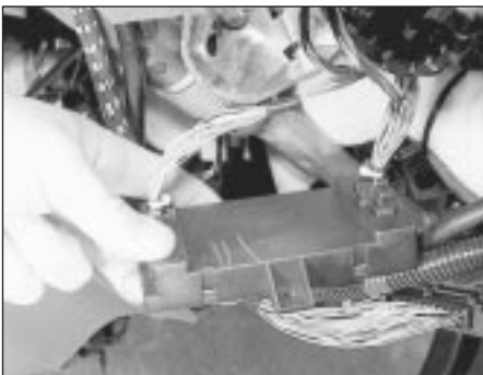
27.27 Removing the auxiliary warning system control module
