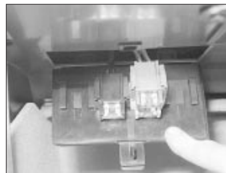
16.3 Auxiliary fuse box in the glovebox
