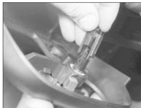
6.22 Removing the switch symbol illumination light
