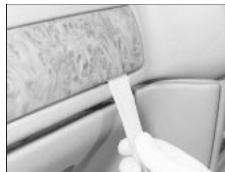
30.18 Carefully prise out the left-hand vent panel . . .
