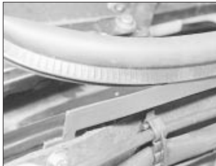
29.2 Pulling off the rubber sealing strip
