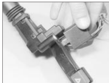
15.19b Unplugging the direction indicator flasher unit
