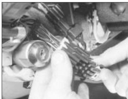
15.19a Disconnecting a steering column switch multi-plug
