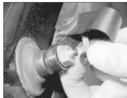
22.7 Disconnecting the rear wiper arm washer hose
