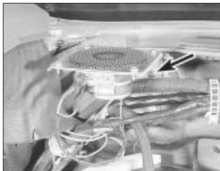
31.15 High frequency loudspeaker located under the fascia top. One bracket securing screw (arrowed) is visible
