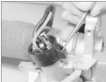
14.3 Ignition/starter switch removal Depress the retaining tabs to lift off the switch
