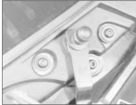
23.2b . . . three screws around the right-hand spindle . . .
