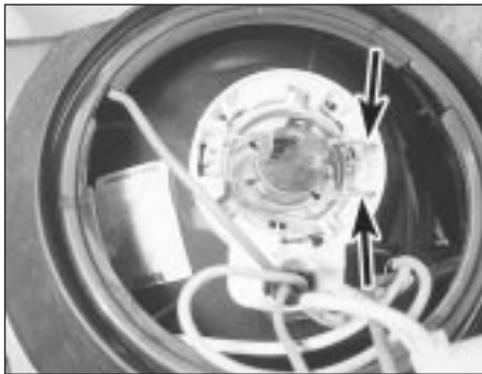
3.2 Squeeze the spring clip legs (arrowed) to remove the headlight bulb
