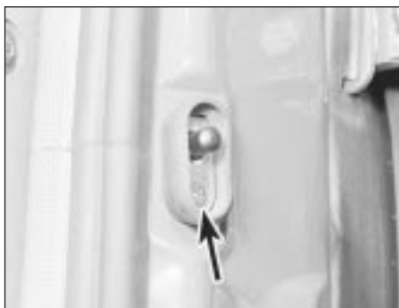
15.24 Door pillar switch securing screws (arrowed)
