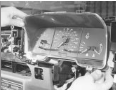
7.4b Removing the instrument cluster
