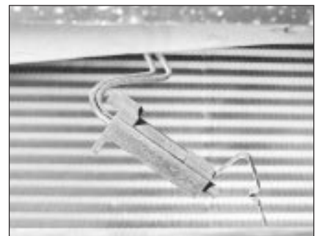
27.9 Removing the air temperature sensor
