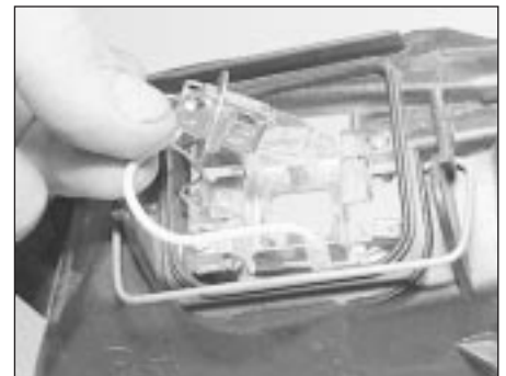
3.10 Removing the auxiliary driving light bulb
