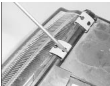
4.9 Removing a headlight lens securing clip
