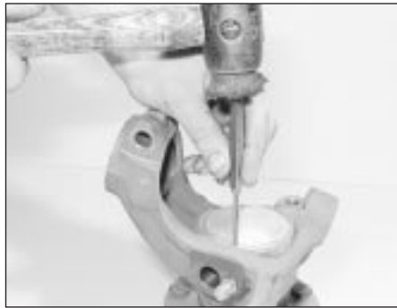
17.17 Seating the new dust cap
