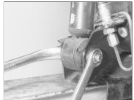
31.5 Undoing a rear shock absorber lower mounting
