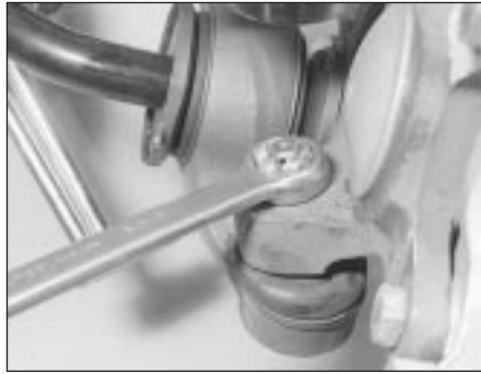
16.4 Slacking the front suspension lower arm balljoint nut
