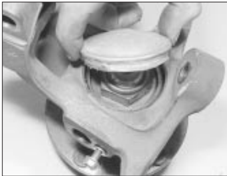
17.3 Removing the dust cap from the stub axle carrier to expose the hub nut
