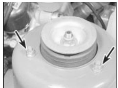
21.8 Two of the three nuts (arrowed) securing the suspension strut to the turret
