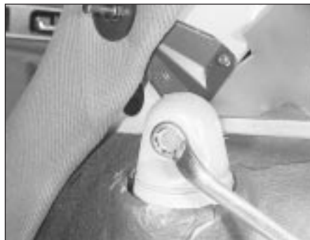
31.4 Undoing a rear shock absorber top mounting
