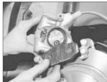
8.5 Removing a rear brake pad
