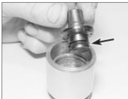
12.4e . . . and the adjuster nut itself Note seal (arrowed) on nut
