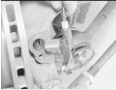
26.3 Removing a front sensor
