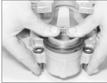
10.9 Pressing the piston into the bore
