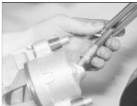
9.5 Removing a front caliper - note clamp on brake hose
