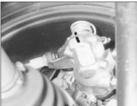
22.4 Alignment marks painted on lever and body
