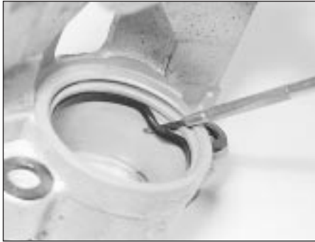
10.5 Removing the piston seal
