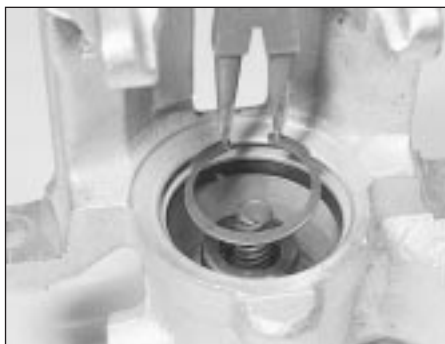
12.7a Extract the circlip . . .
