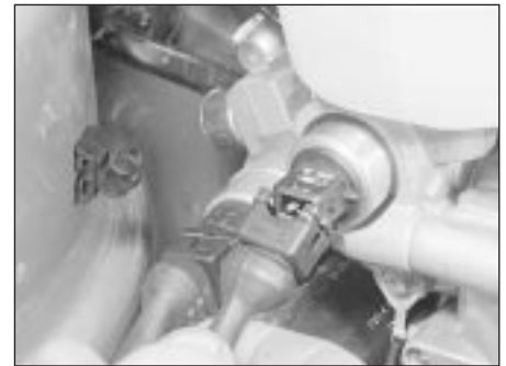
15.3c Disconnecting the main valve plug
