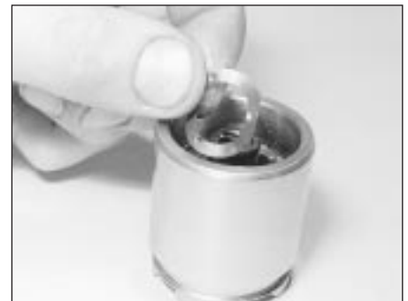
12.4c . . . a wave washer and (not shown) another thrustwasher . . .
