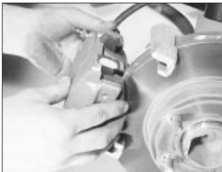
7.5 Lifting a front caliper off the disc
