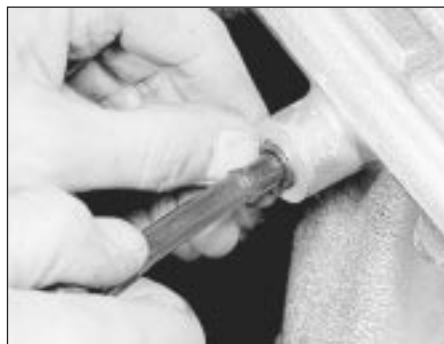
29.2 Disconnecting brake servo vacuum hose from the inlet manifold (DOHC engine shown)
