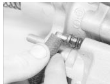
16.5b . . . and disconnect the hose
