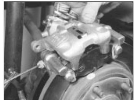
11.5b . . . and remove the rear caliper
