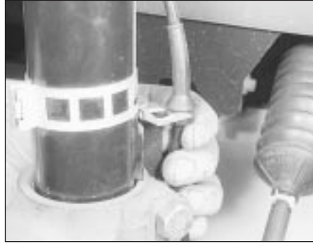
26.4 Unclipping the sensor wire from the strut
