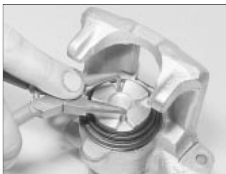
8.7 Rotating the caliper piston to retract it
