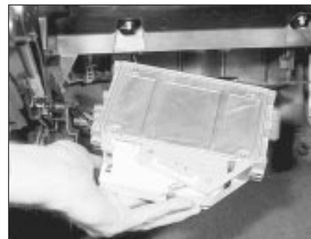
31.4 Removing the ABS control module - models from April 1992
