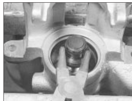
12.6 Using the adjuster nut to compress the caliper spring
