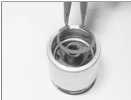
12.4a Removing the circlip from a rear caliper piston . . .
