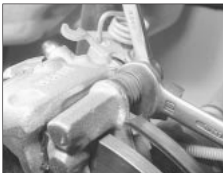
8.3 Undoing a rear caliper front slide bolt
