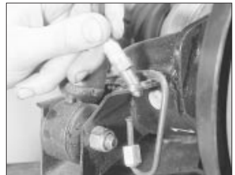
21.4 Removing a flexible hose from its bracket
