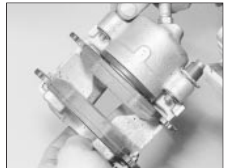
7.8b Both pads fitted to a front caliper
