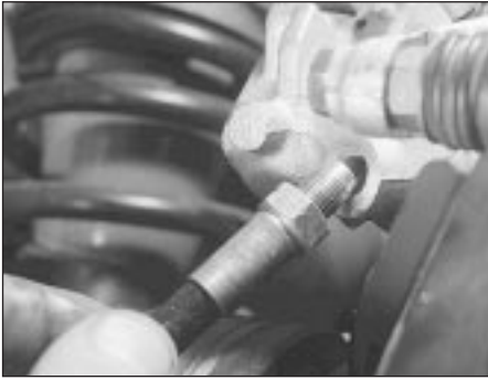
21.5 Disconnecting the hose from the caliper
