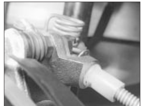
23.4 Handbrake cable outer attached to caliper bracket
