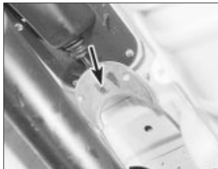
23.3 Circlip (arrowed) on equaliser yoke Note protruding screws in transmission tunnel
