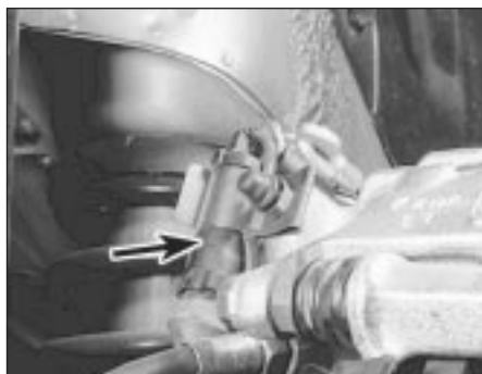
8.4 Pad wear warning multi-plug (arrowed) on rear caliper
