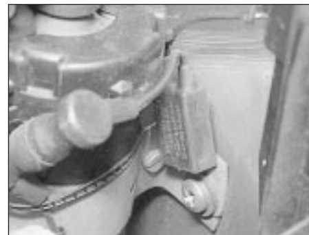
16.6 Suppressor secured by one of the coil retaining screws
