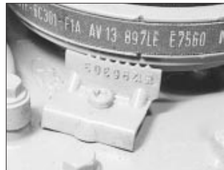
13.20 Crankshaft pulley notch set to the 12° BTDC position
