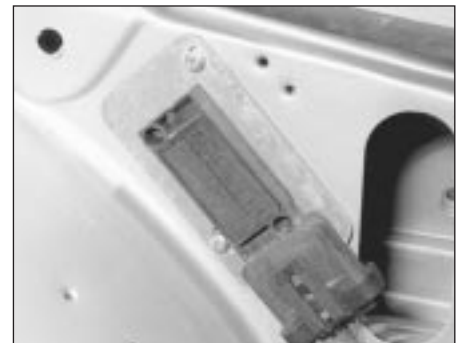
15.15 Ignition module (viewed with air cleaner removed)
