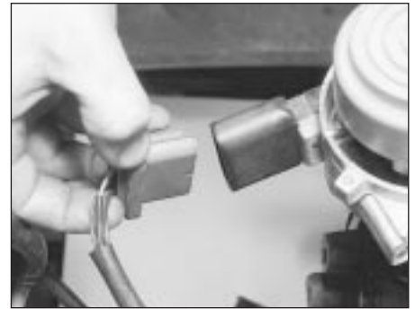
13.5 Disconnecting a distributor multi-plug
