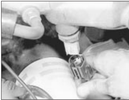
20.4 Coolant temperature sensor multi-plug
