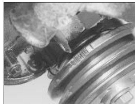
14.3a Timing marks and pointer Cast pulley shown
