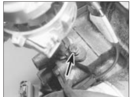
13.6 Distributor clamp bolt (arrowed)
