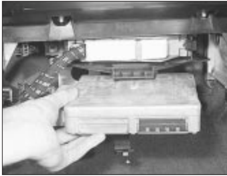
18.15 Removing the engine management modules (glovebox removed for clarity)
