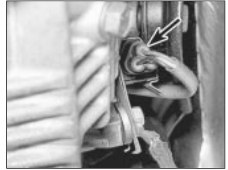
27.4 Vehicle speed sensor wiring plug (arrowed)
