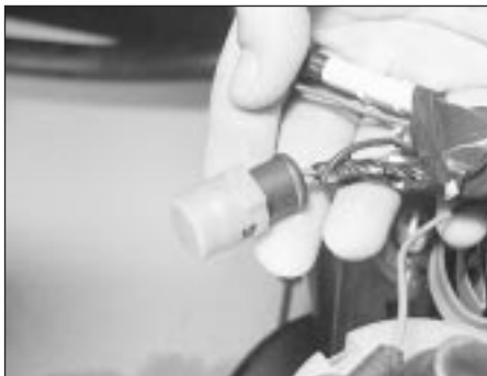
23.2a Octane adjustment lead multi-plug
