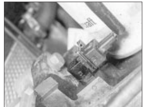
24.1 Crankshaft speed/position sensor (viewed from underneath)
