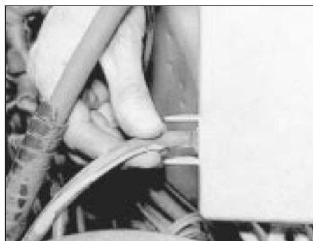
18.2 Disconnecting the ESC II module vacuum pipe
