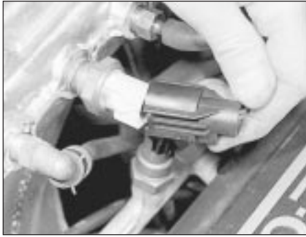
25.3 Disconnecting the air charge temperature sensor wiring plug
