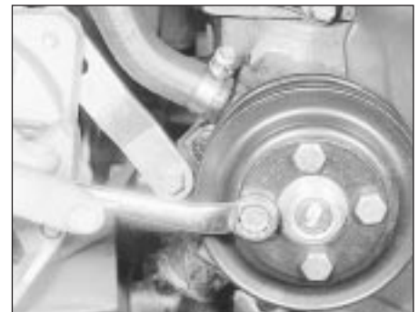
11.4 Undoing a water pump pulley bolt
