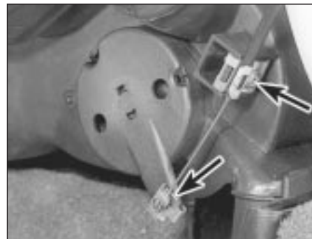
18.19 Heater control cable retaining screw and clip (arrowed)
