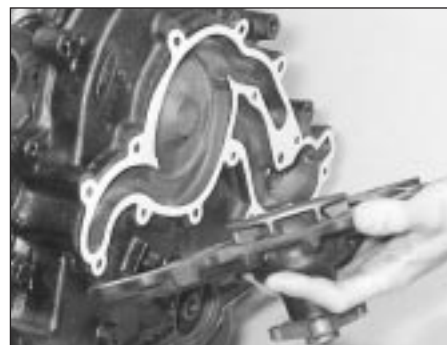
11.28 Removing the water pump
