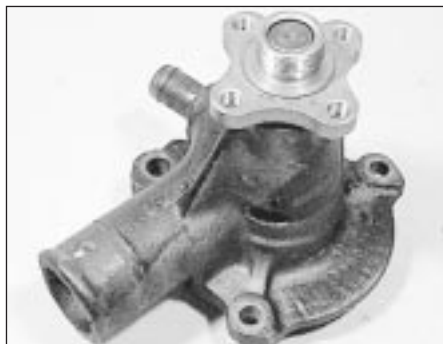
11.7b Water pump removed
