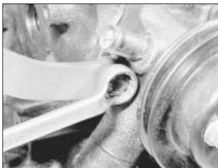
11.7a This water pump bolt also secures the alternator strap
