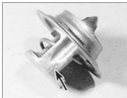
7.7 Thermostat direction of flow arrow
