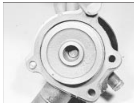
11.9 Fitting a new gasket to the water pump
