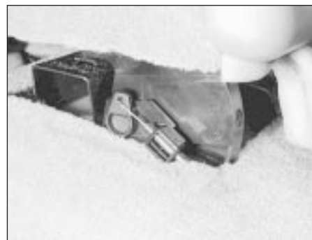
18.14 Rear heater control cable at nozzle
