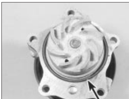
11.18 On refitting, renew the water pump O-ring (arrowed)
