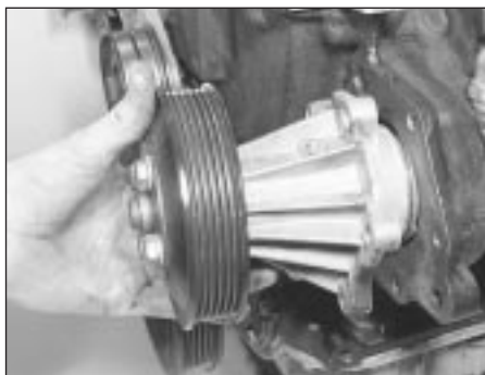
11.17 Withdrawing the water pump from the cylinder block (engine removed)
