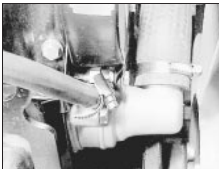
7.3 Top hose attachment to the thermostat housing
