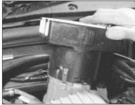
39.6 Removing a distributor screening can - V6 engine
