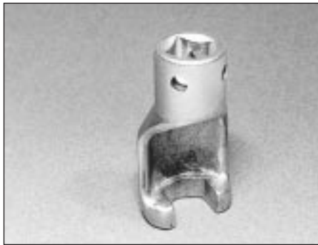
23.11 Cutaway socket spanner
