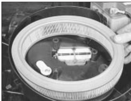
38.3 Removing the air cleaner element (carburettor model)
