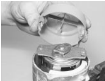
39.9 Removing a rotor arm
