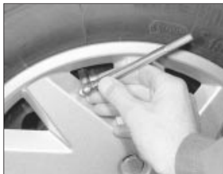
4.3 Checking tyre pressure
