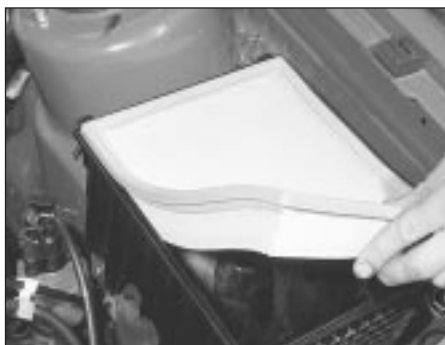
38.11 Removing the air cleaner element (fuel-injection SOHC and V6)
