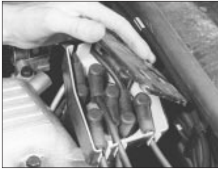
39.3 Removing a distributor can screening lid - V6 engine
