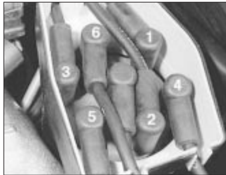
39.17 HT lead identification at distributor cap - V6 engine
