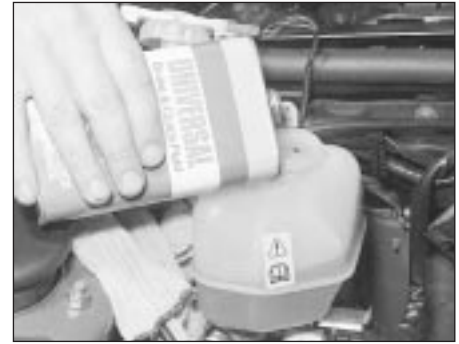
3.15 Topping up the brake fluid reservoir
