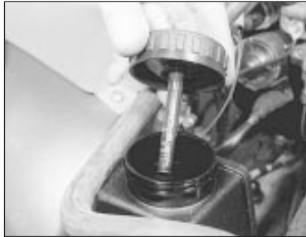
35.2 Removing the power steering fluid dipstick
