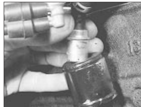
42.1 Pulling the vent valve from the oil separator - SOHC engine
