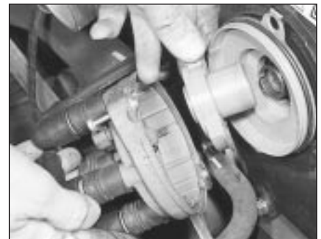
39.24 Removing the distributor cap and rotor arm - DOHC engine
