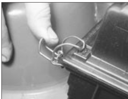
38.9 Air cleaner cover spring clip (fuel-injection SOHC and V6)
