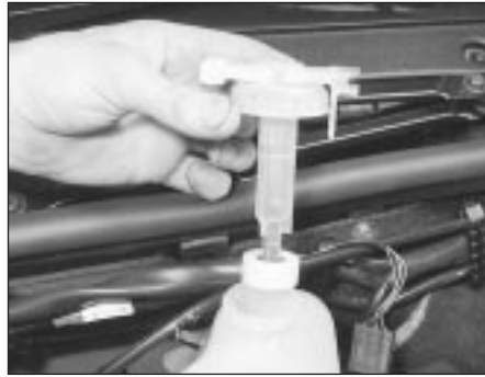
3.14 Removing the brake fluid reservoir cap
