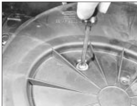
38.1 Removing an air cleaner cover screw (carburettor model)
