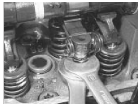
23.9 Adjusting a valve clearance - SOHC engine
