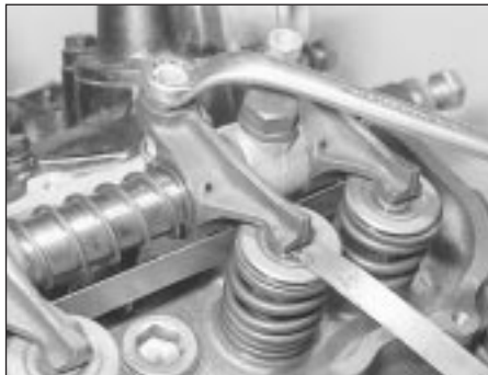
23.20 Adjusting a valve clearance - V6 engine
