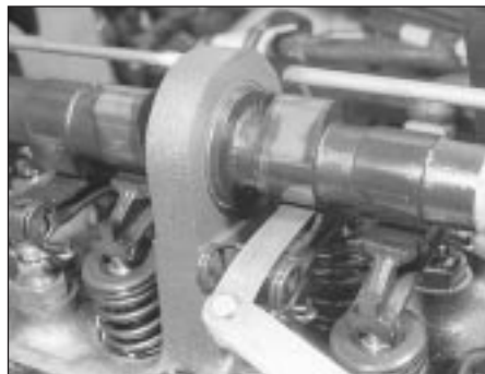
23.7 Measuring a valve clearance - SOHC engine
