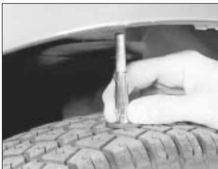
4.1 Checking the tyre tread depth
