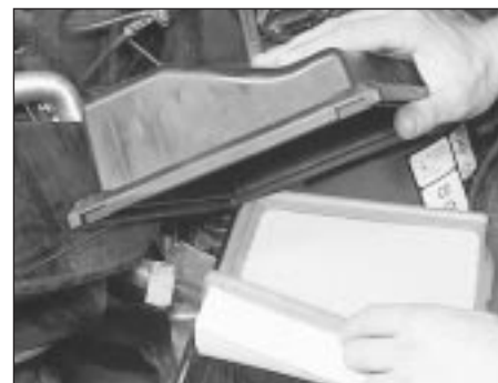
38.19 Removing the air cleaner element (fuel-injection DOHC)
