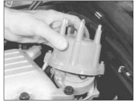
39.7 Removing a distributor cap
