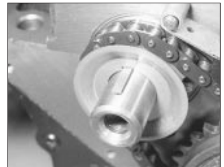
15.15 Fit the oil slinger with its convex side against the sprocket
