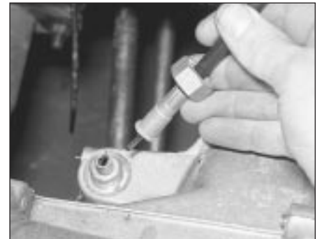
11.50 Disconnecting the speedometer cable - HCS engine
