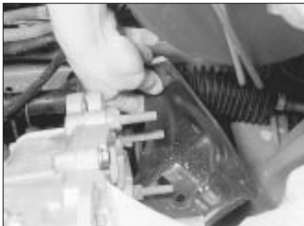
11.65b Removing the mounting bracket - HCS engine
