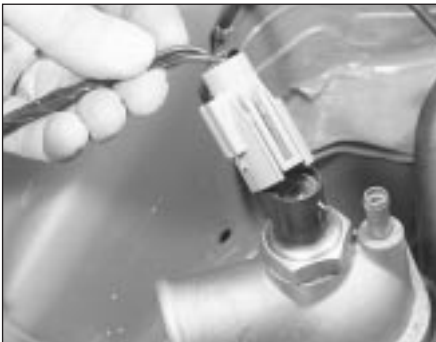
11.49a Disconnecting the cooling fan thermal switch . . .
