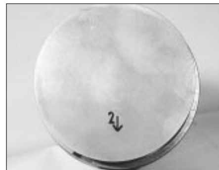
8.13b Arrow on piston crown must face the timing cover when installed
