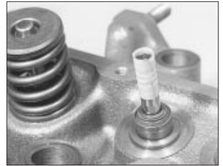
14.14c Tape the end of the valve stem before fitting the valve stem seal - HCS engine
