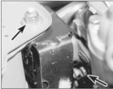
11.57a Right-hand engine mounting nuts/bolts (arrowed) - HCS engine
