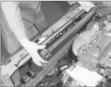
11.41c Lifting out the radiator - HCS engine
