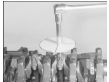
15.43d . . . and using a card template to angle-tighten the big-end cap bolts - HCS engine
