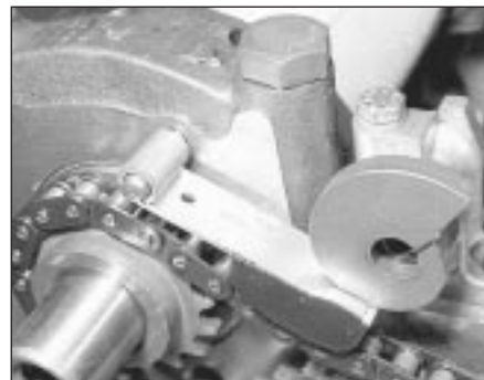
15.14 Refit the timing chain tensioner and arm
