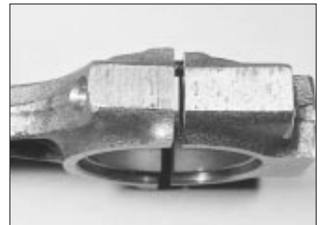
12.37 Connecting rod and big-end cap markings
