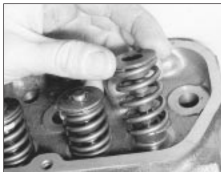
13.39 Remove the valve spring retainer and spring . . .
