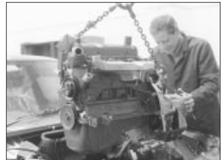
11.66b ... and out of the engine compartment
