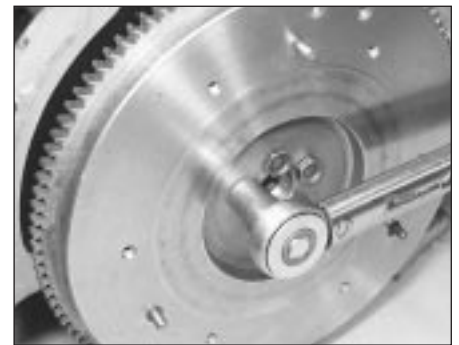
15.18b . . . then refit and secure the flywheel
