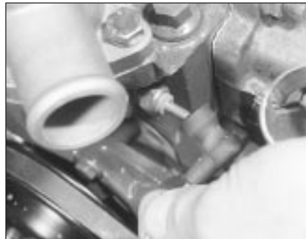
11.49b . . . and coolant temperature sender - HCS engine
