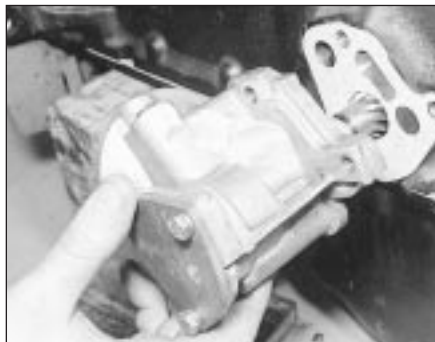
10.3 Removing the oil pump
